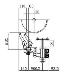
"X" = the tensile axis, the length must be at least 90 mm.
